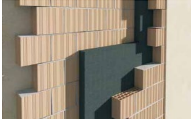
Thermal and acoustic insulation
